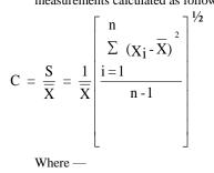
$X_i$ = ith measurement  $\overline{X}$  = mean value of measurements S= estimated standard deviation n= number of measurements;
