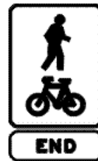
End shared path sign
