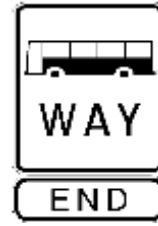
End busway sign
