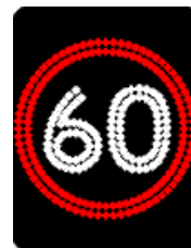
Speed limit sign (Variable illuminated message sign) (circle illuminated red)
