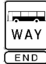
End busway sign
