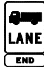
End truck lane sign
