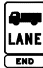
End truck lane sign
