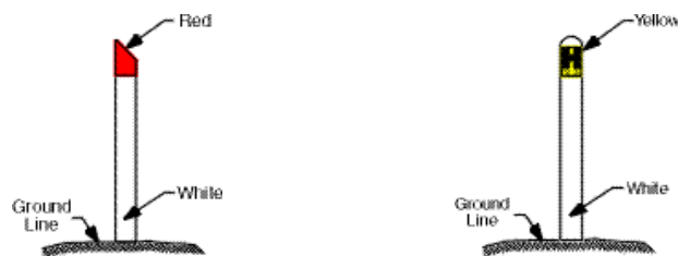
Fire hydrant indicators
