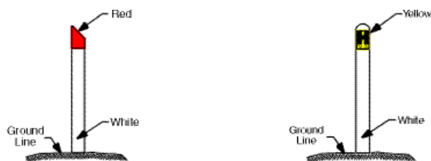
Fire hydrant indicators
