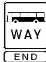
End busway sign
