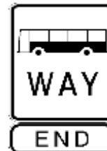
End busway sign
