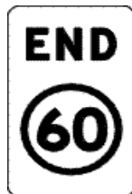
End speed limit sign
