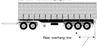
Tow coupling overhang Tow coupling overhang — dog trailer
