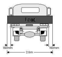
Vehicle loaded to width limits mentioned in r. 170, with maximum side projection of load allowed under r. 180
