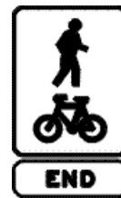
End shared path sign
