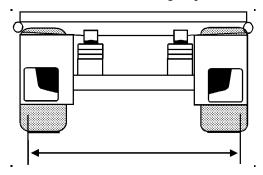
Ground contact width of an axle
