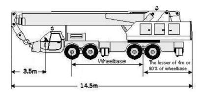
Rigid mobile crane, showing dimension limits
