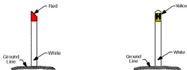
Fire hydrant indicators
