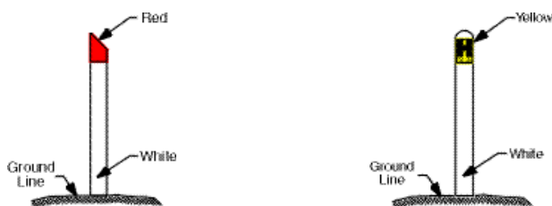
Fire hydrant indicators
