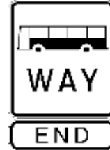
End busway sign
