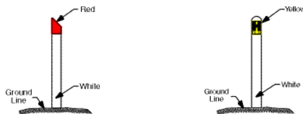
Fire hydrant indicators
