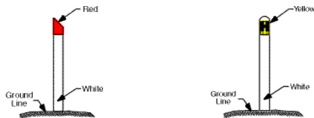
Fire hydrant indicators
