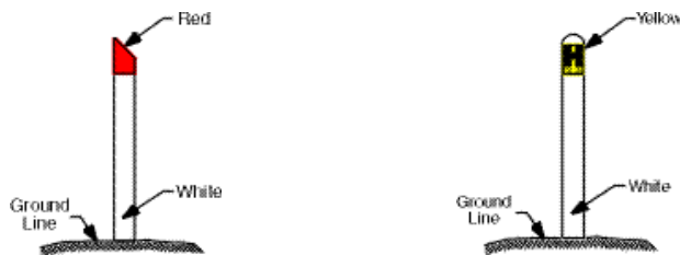
Fire hydrant indicators
