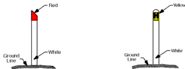
Fire hydrant indicators
