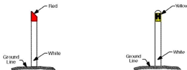
Fire hydrant indicators
