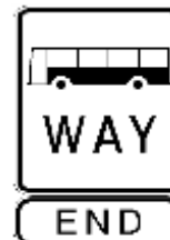
End busway sign
