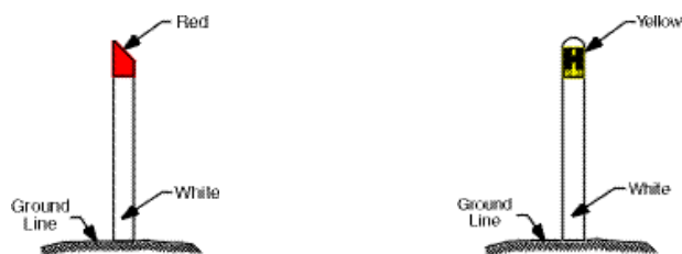
Fire hydrant indicators
