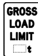
Gross load limit sign
