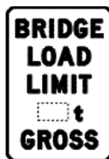
Bridge load limit (gross mass) sign
