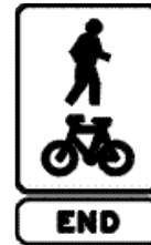
End shared path sign
