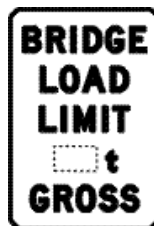
Bridge load limit (gross mass) sign
