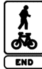
End shared path sign
