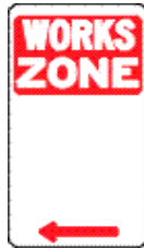
Works zone sign (arrow and background to words in red)
