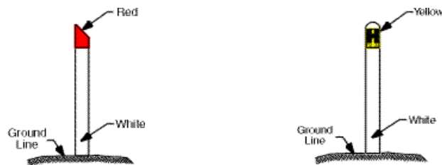
Fire hydrant indicators
